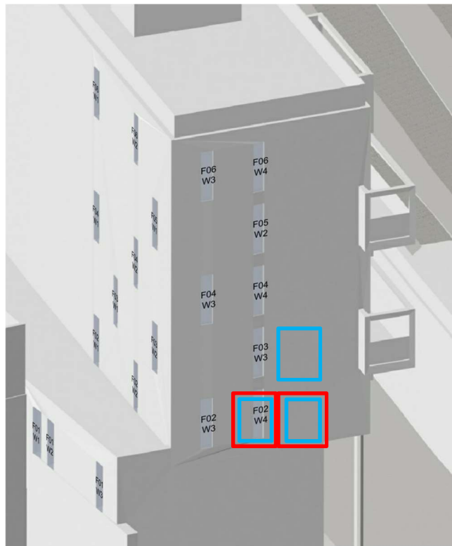
Image 20 (above): Model showing the affected windows in terms of VSC in red and affected windows in terms of NSL in blue
